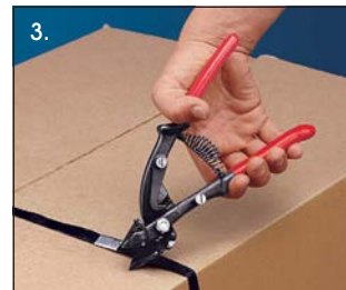
3. CUTTER Cuts excess strapping.
